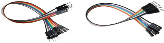
Fig 3.12(a): Female to Male Jumper Wire. Fig 3.12(b): Male to Male jumper
