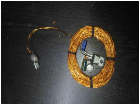
Figure 5.2: Imbedded Coils or receiver coil
