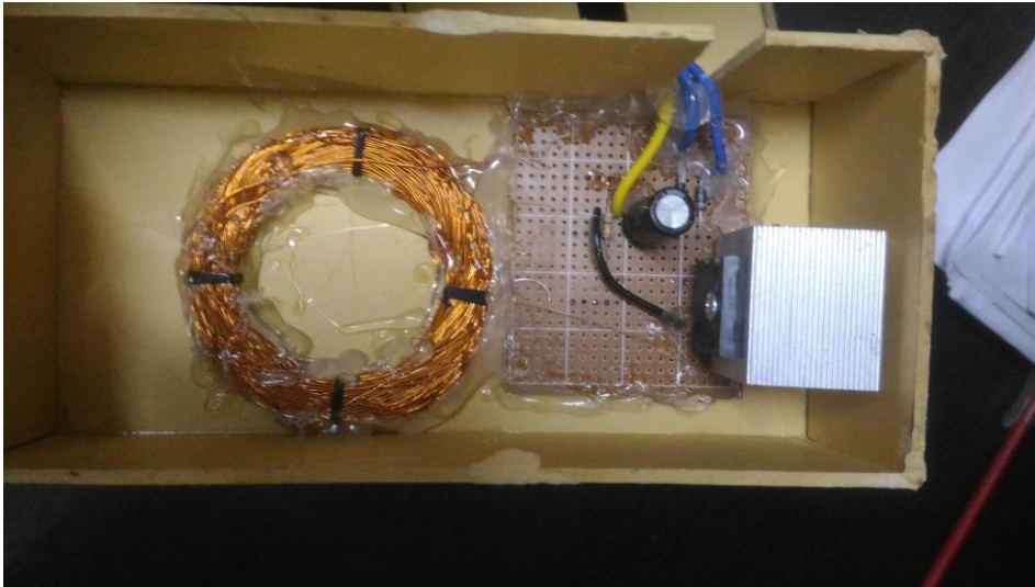
Figure 5.1: Primary coil & main circuit board
