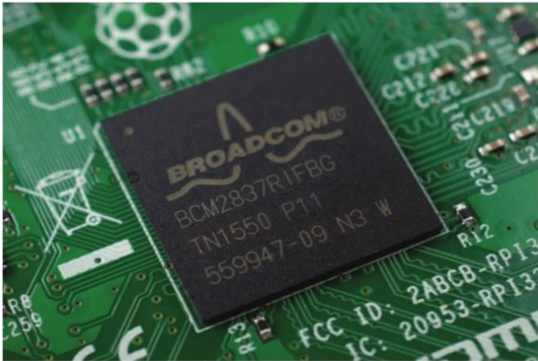
Figure 2: System on Chip Broadcom BCM2837 [3]
