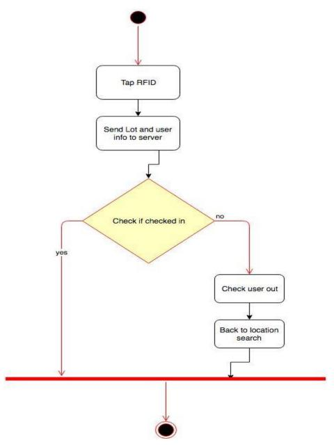
Figure 3.5: Check-out diagram
