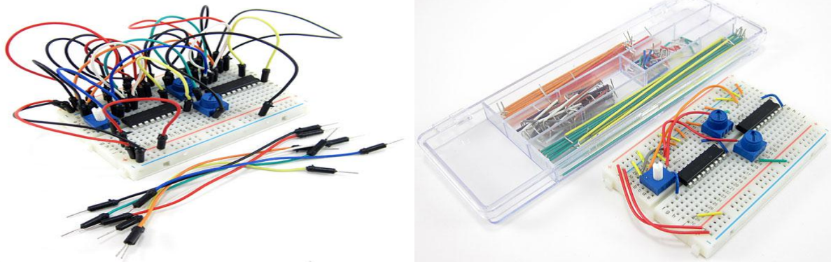
Fig 3.15: Flexible jumper wires
