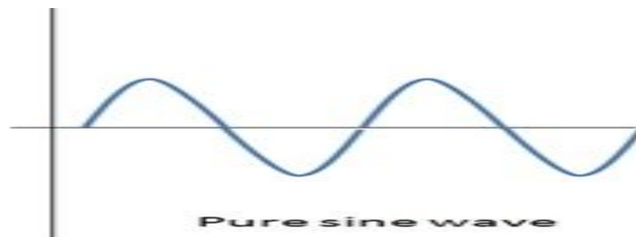
Figure 3.4: Output of a Pure Sine Wave Inverter
