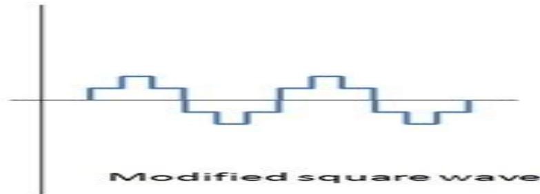
Figure 3.2: Output of A Quasi-Square Wave Inverter
