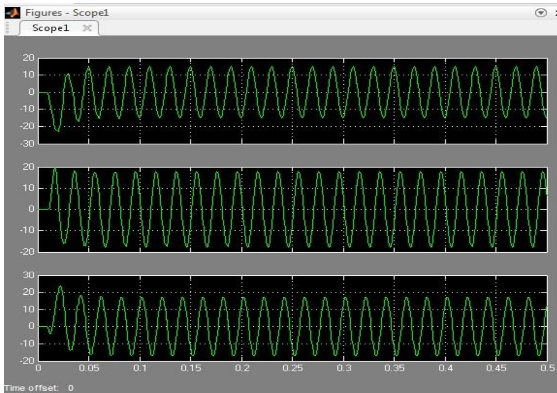
Figure4.1: Mat Lab Simulation Output for Current (a. Phase 1, b. Phase 2, c. Phase 3)
