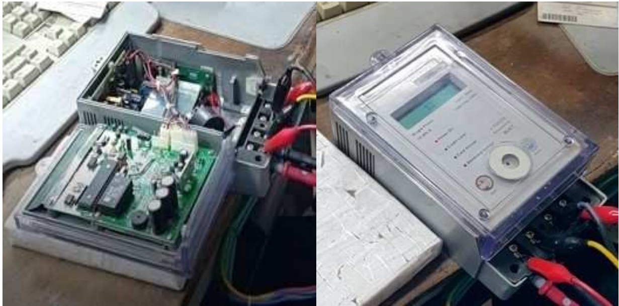
Figure 7.8: Prepaid Meter (a) outside view, (b) inside view.
