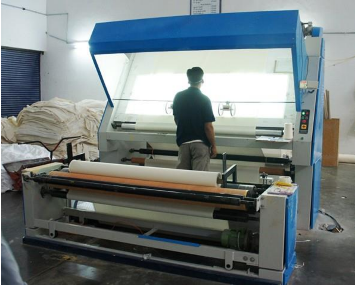
Figure: Fabric Inspection Machine.
