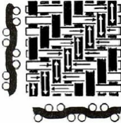
Figure 25: Movement of yarn in twill fabric
