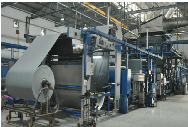
Figure 8.6: Finishing Machine used in ADML (Sanforizing & stenter)
