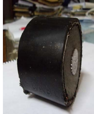
Figure 5.11: XLPE insulated Underground Power Cable used in APSCL
