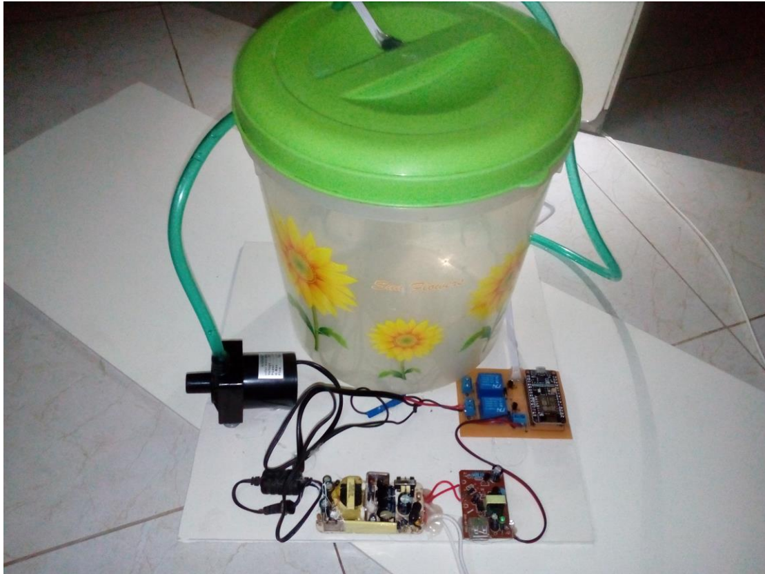
Figure C6: Automated water management system for smart home
