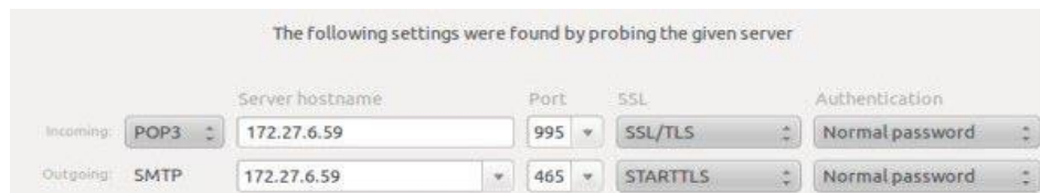
Figure 3.17: Shows Screen Print POP3 and SMTP host and Port configuration
