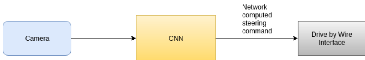
Figure 3.4.2.1: Nvidia's The trained network is used to generate steering commands from a single front-facing camera
