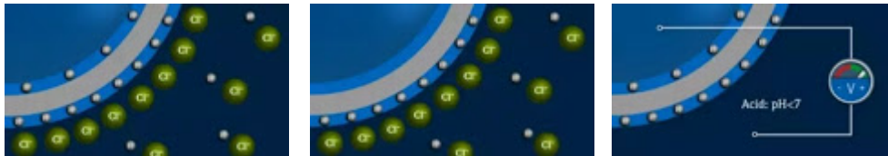
Fig1.1: How pH meter works
