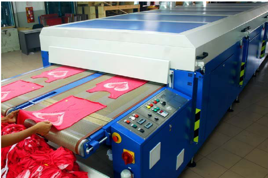
Fig:3.10 Automatic Screen Printing & Curing/Ageing
