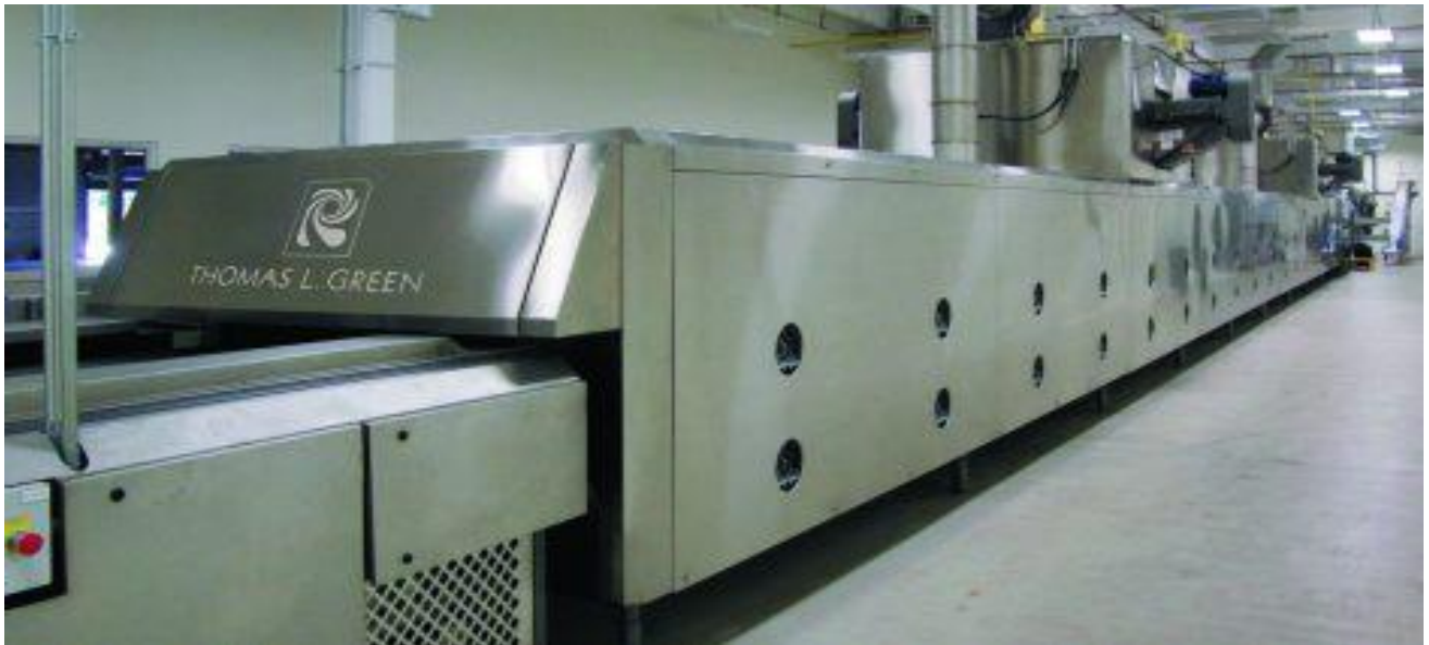
Figure: gas chamber oven
