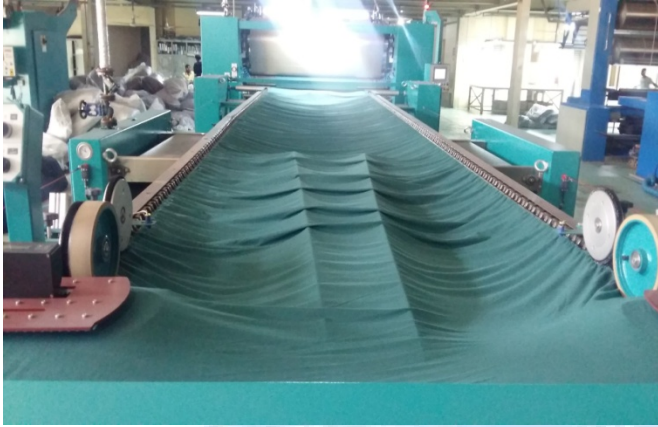
Photo: Compactor machine
