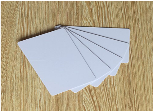
Figure 3.9: RFID security door lock unbelted card
