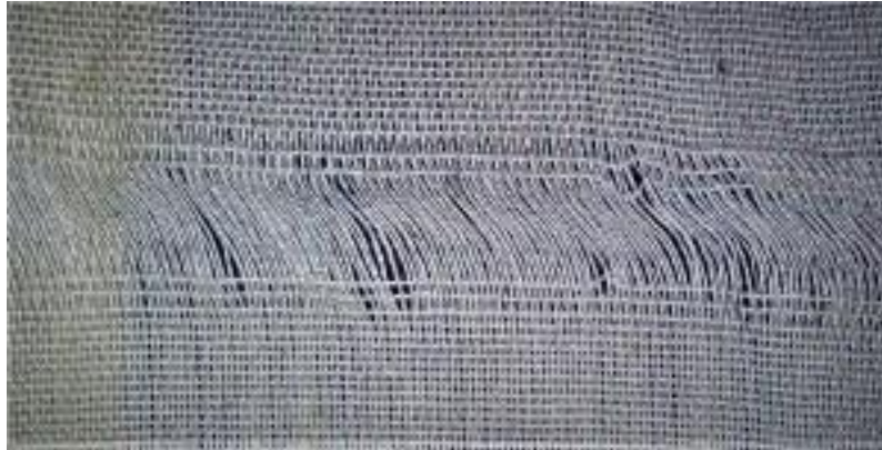
Figure3.1: Crack between stripes
