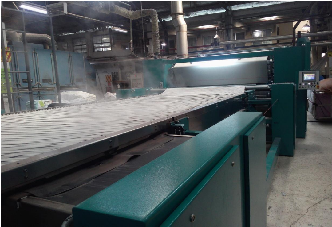
Open Compacting M/C
