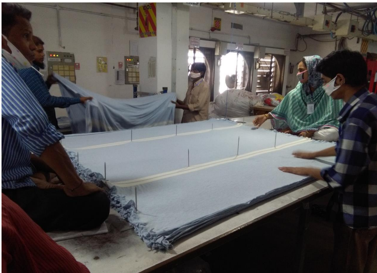
Figure 3. 6: Fabric spreading by manually
