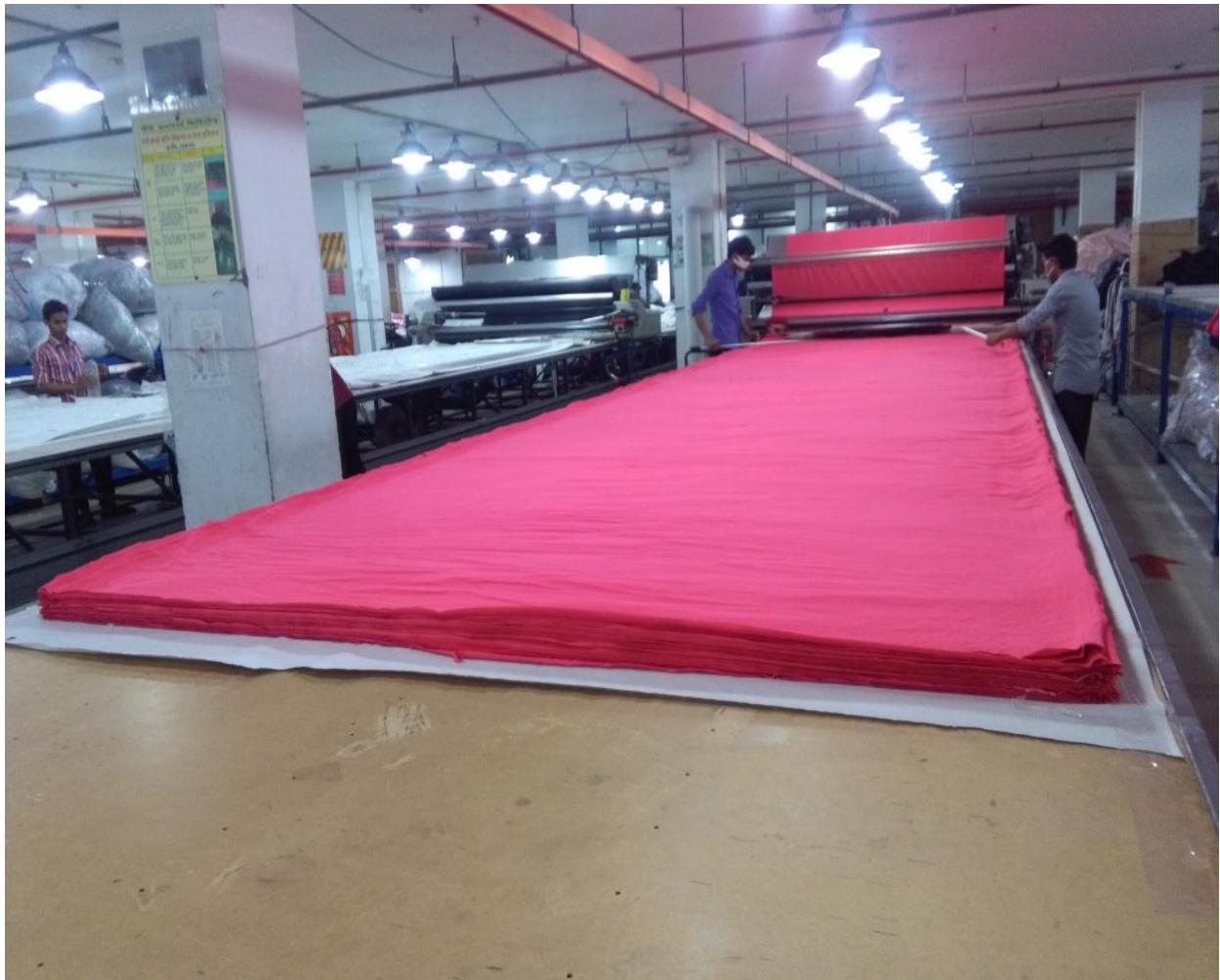
Figure 3. 7: Fabric spreading by mechanical method
