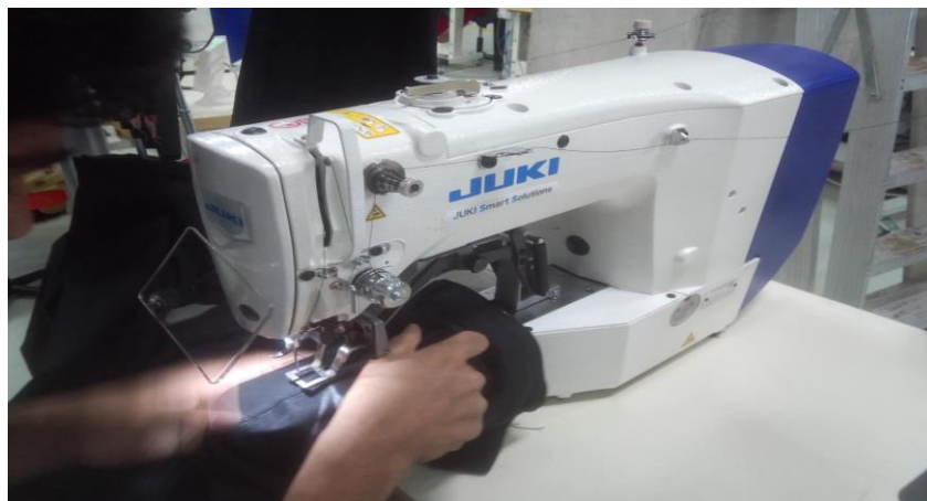
Figure: Bar tag lock stitch Machine.
