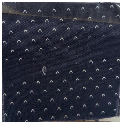
Figure -8: DYE DEFECT
