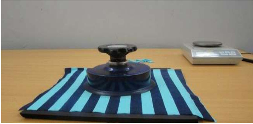
Fig2.5: GSM Cutter for Fabric GSM Checks
