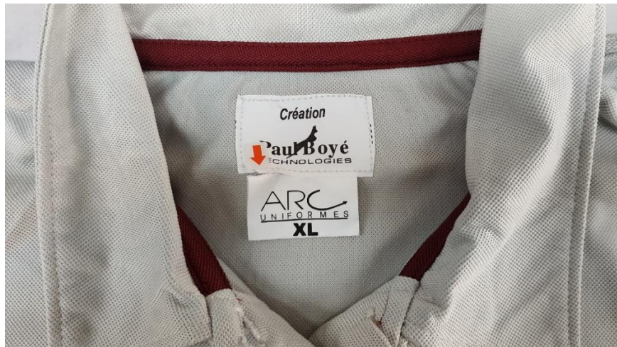
Figure 3.3.6.11 Improper Size Label Joining
