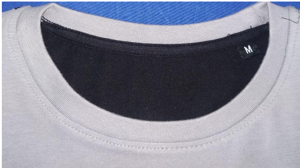
Figure 3.3.6.4 Main Label Missing
