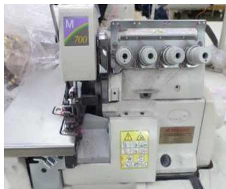
Fig 17: Over lock machine
