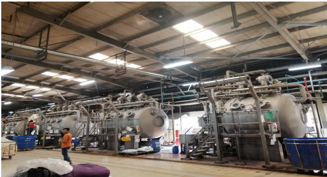
Fig 12: Thies Dyeing machine
