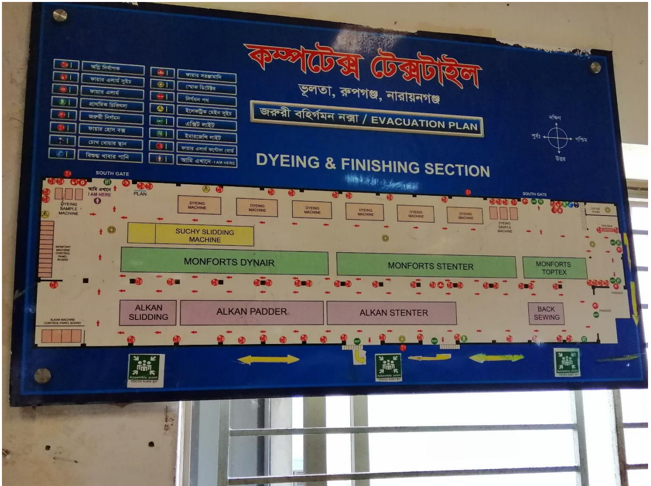
Fig 11: Lay out of Dyeing & Finishing
