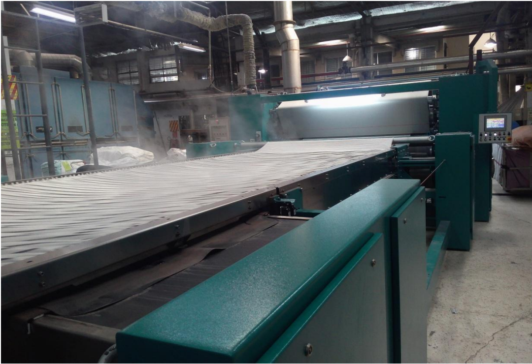
Open Compacting M/C
