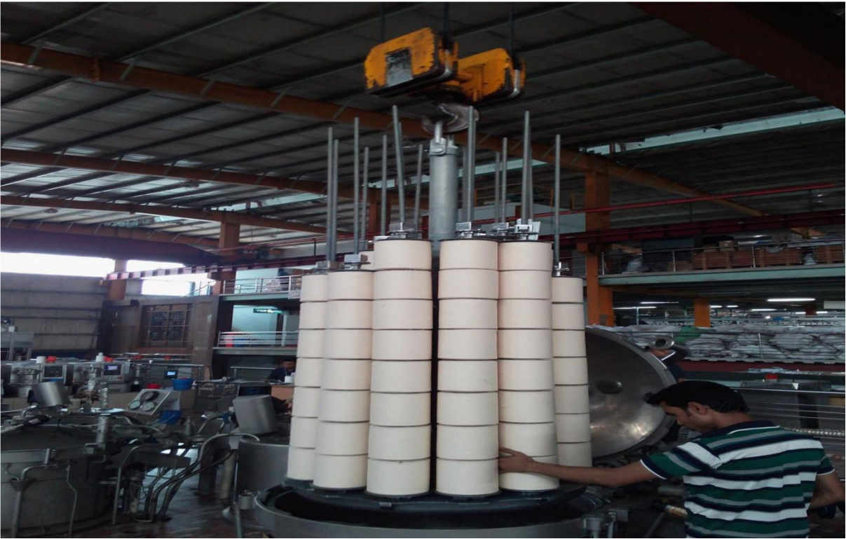
Package Loading on Bulk Machine
