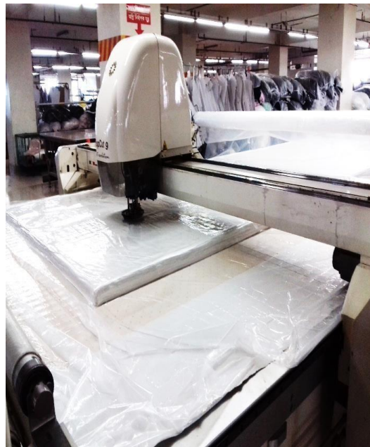
Figure 3.7: Auto Fabric Cutter
