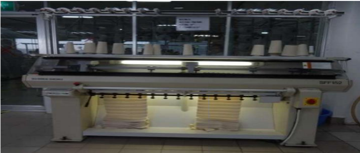
Figure 3.25: Flat knitting Machine
