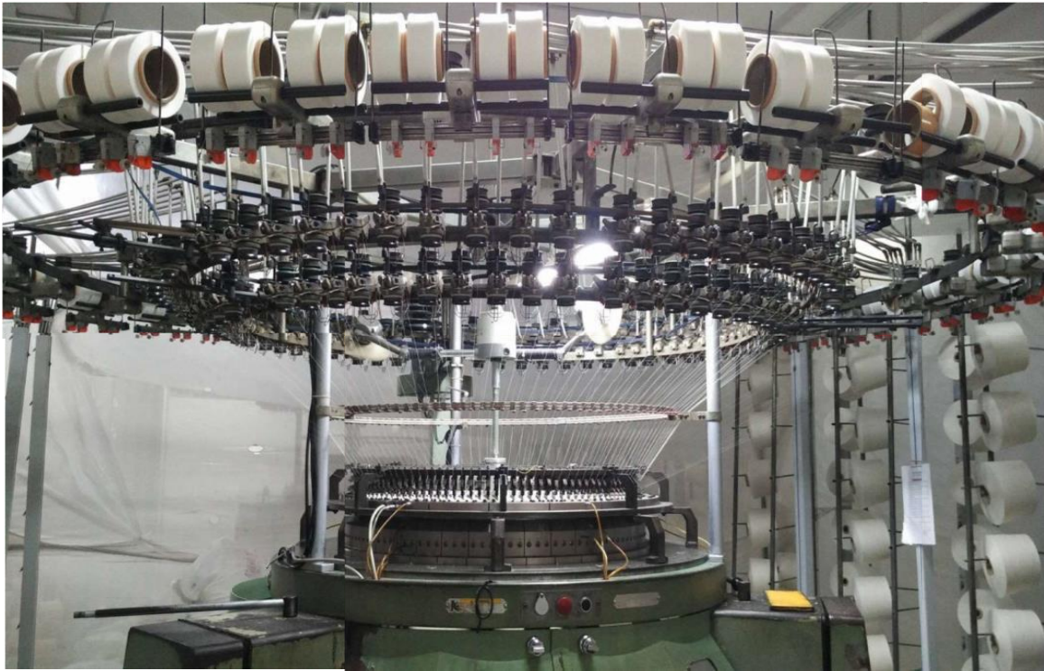
Figure 3.24 : Circular Knitting Machine
