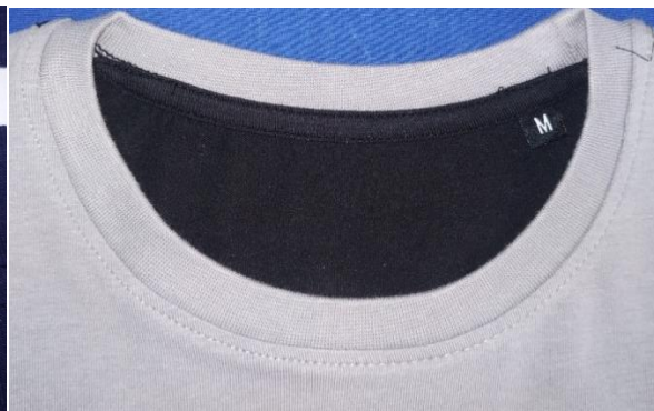
Figure 3.1.3: Main Label missing
