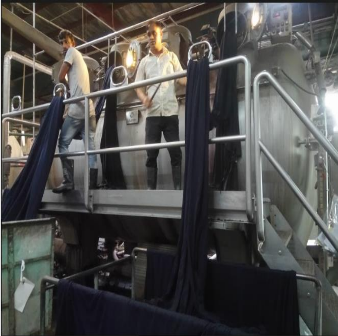
Fig.3.26: Shade check and inspection
