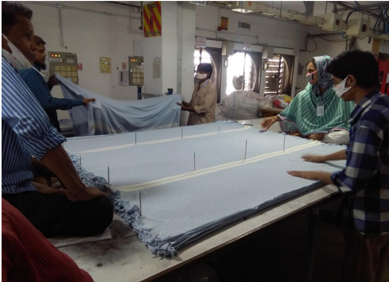
Figure: 3.3.1 Fabric spreading by manually
