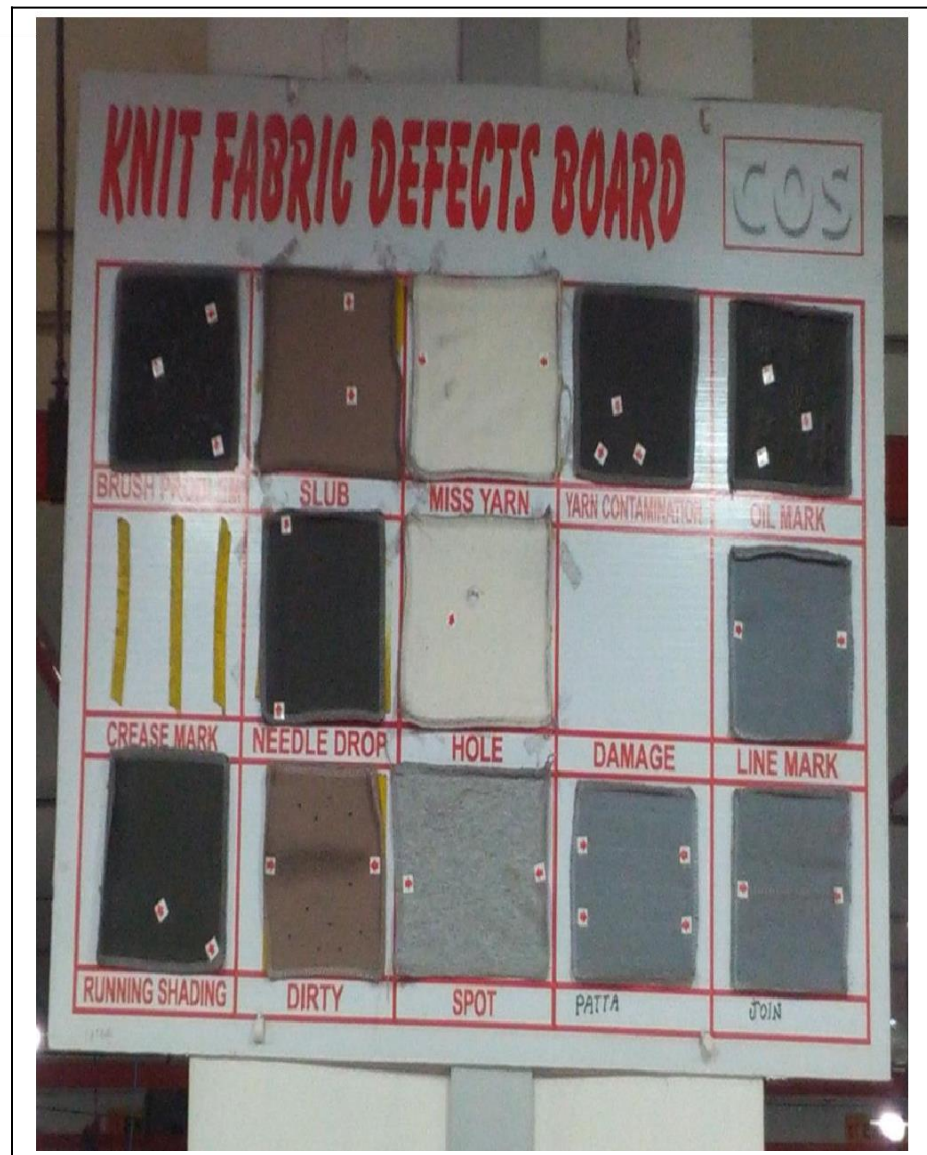
Figure: 3.3.5 Fabric Fault
