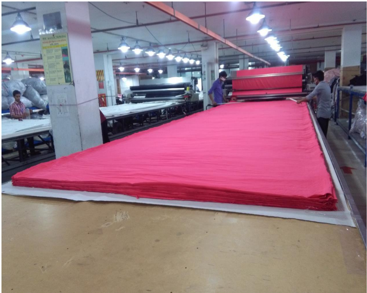
Figure: 3.3.2 Fabric spreading by mechanical method
