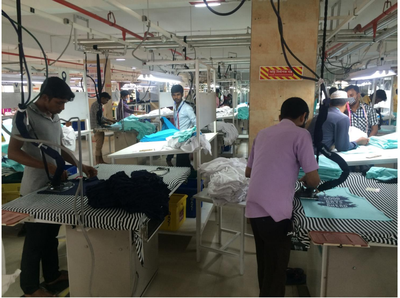
Fig: 3.4.4.2 Steam iron m/c
