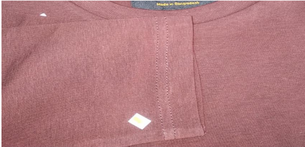
Figure 3.3.6.6 Chap Tuck Missing
