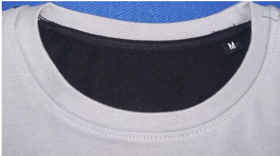
Figure 3.3.6.4 Main Label Missing
