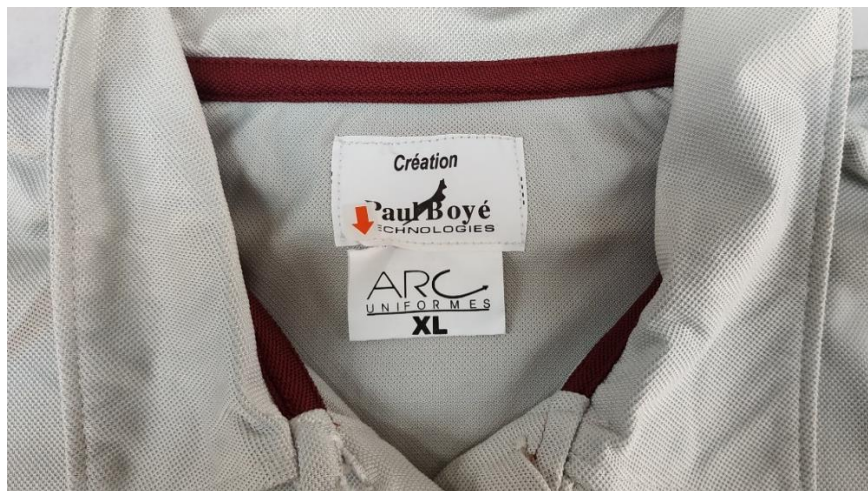
Figure 3.3.6.11 Improper Size Label Joining
