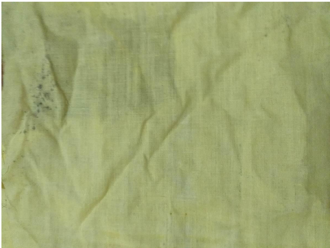
After applying 3Mpa pressure (3 times) rubbing fastness is 4 out of 5
