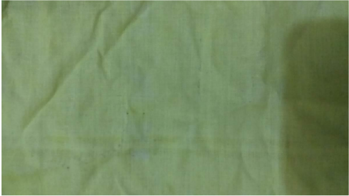
After applying 3Mpa pressure (2 times) rubbing fastness is 2/5 out of 5
