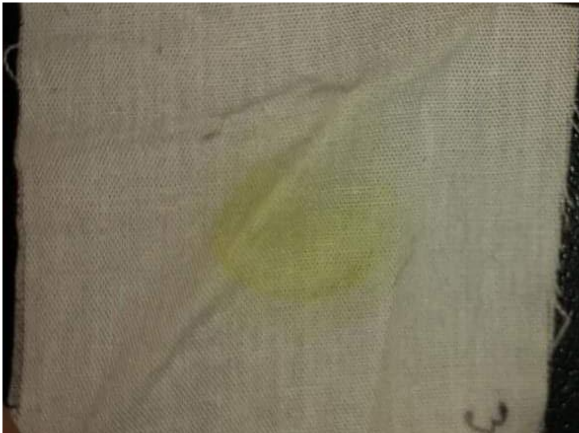
After applying 3Mpa pressure (2 times) rubbing fastness is 2/5 out of 5
