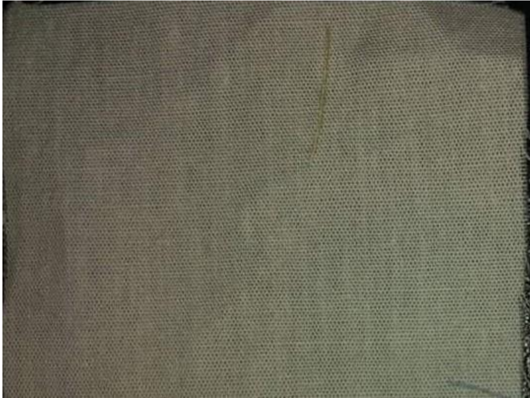
After applying 3Mpa pressure (2 times) rubbing fastness is 4 out of 5
