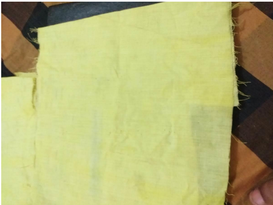
After applying 5Mpa pressure (1 time) rubbing fastness is 4/5 out of 5
