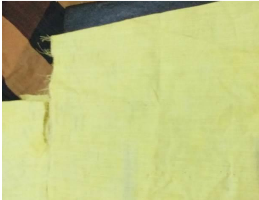
After applying 5Mpa pressure (1 time) rubbing fastness is 3 out of 5
