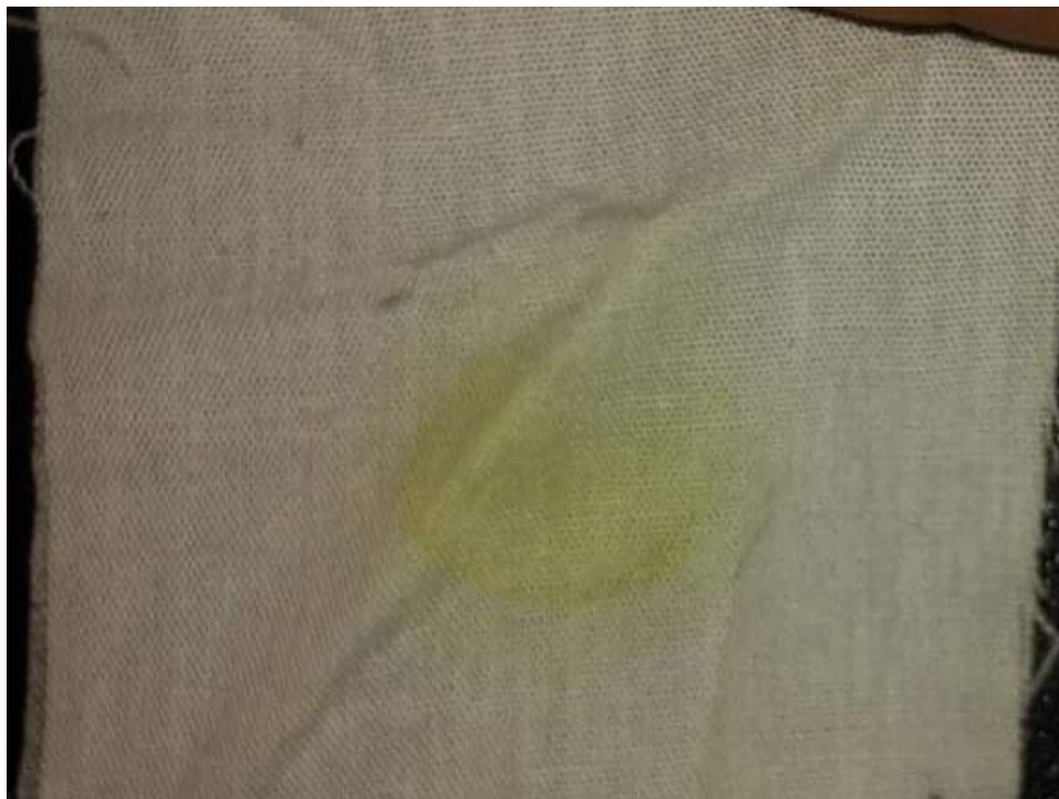
After applying 5Mpa pressure (1 time) rubbing fastness is 3 out of 5
