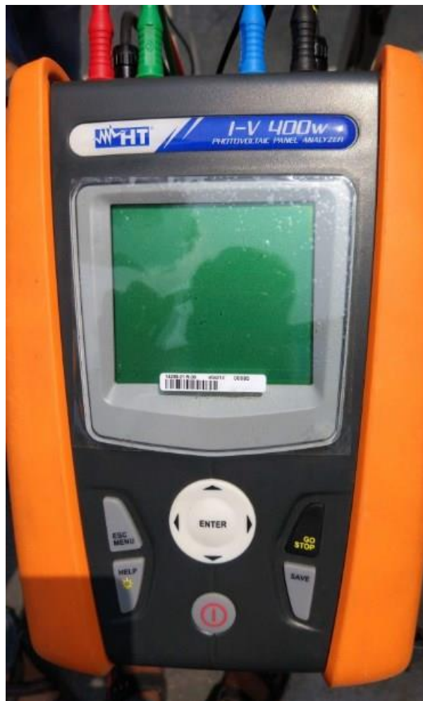
Figure 4.5: I-V 400 W Photovoltaic Panel Analyzer.
