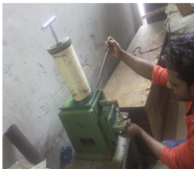
Fig: 3.27. Top Roller arbor greasing.
