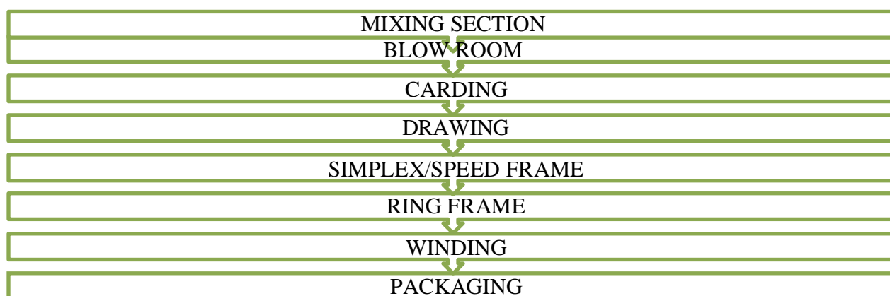
FIG.2.1. Process Flow Chart of Spinning
