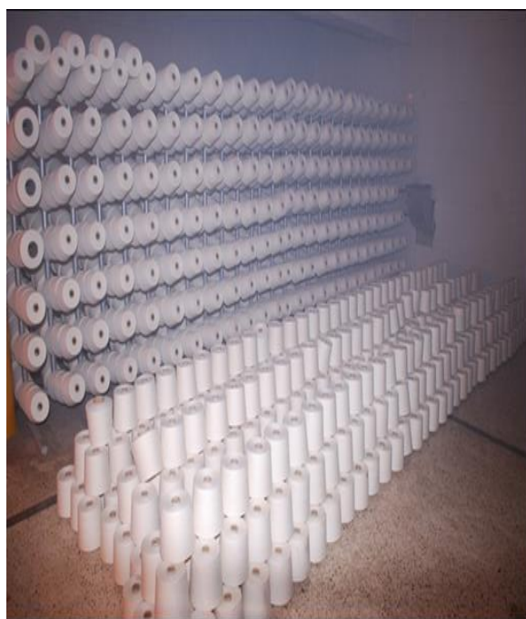
Fig: 2.22. Yarn packaging of Cone form.
