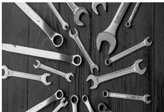
Fig: 3.12. (Combination Tools (Spanners): Tightening and loosening of nuts & bolts.
