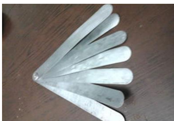
Fig: 3.9. Leaf gauge for Card setting.
