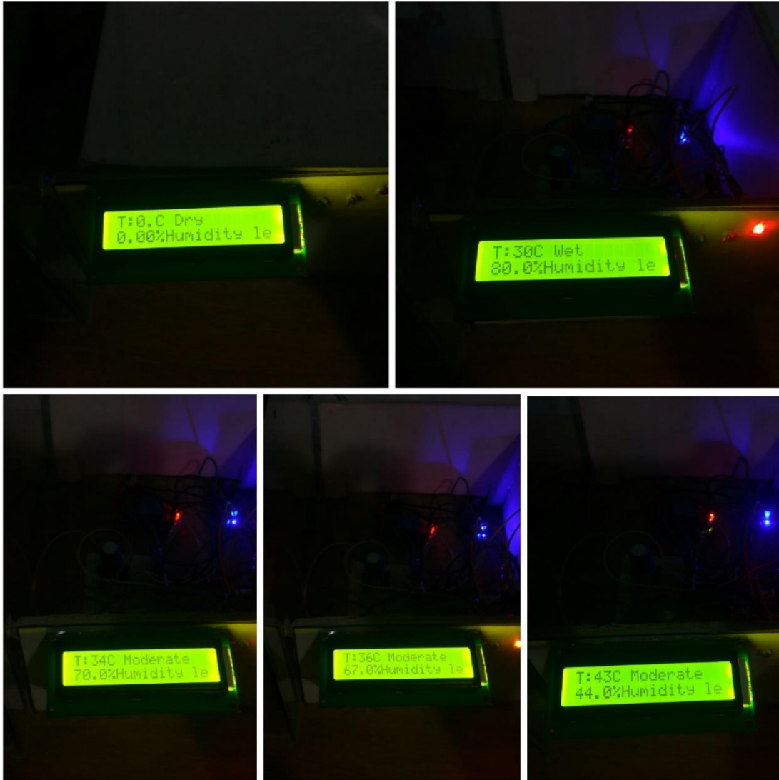
Figure 5.4: Output of Temperature and Humidity
