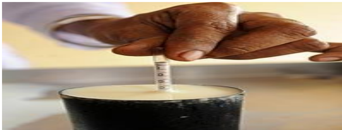
Figure: Corrected Lactometer Reading test
