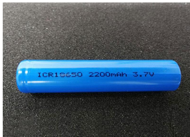
Fig 3.3: Battery – Lithium-ion battery
