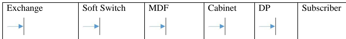
Figure 2.2: BTCL Communication Structure
