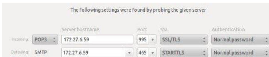
Figure 3.3.17: Shows Screen Print POP3 and SMTP host and Port configuration
