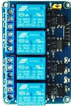
Fig: 4.7 Image of our 4 channel Relay module.
