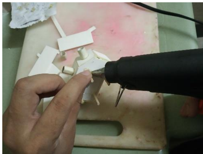
Figure: 5.1.9.36 Attaching (pvc board) parts using hot glue
