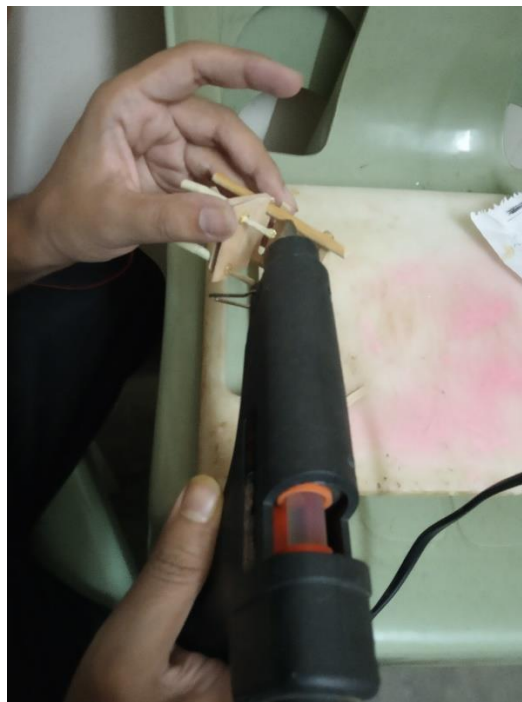
Figure: 5.1.9.46 Chair parts attaching using hot glue
