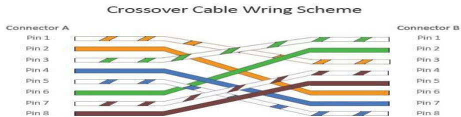
Figure:3.15 Crossover Cables.
