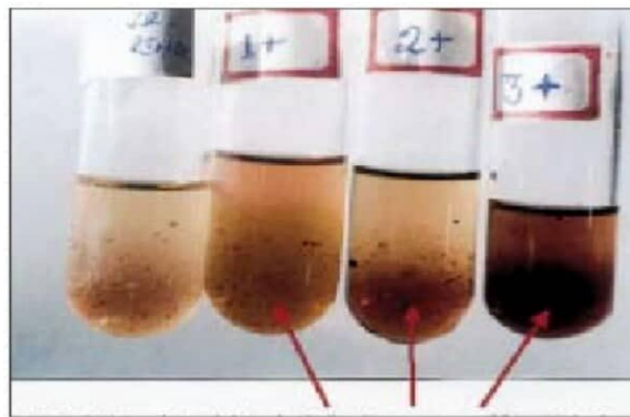
Figure 1: Red purple to violet color indicating presence of formaldehyde
