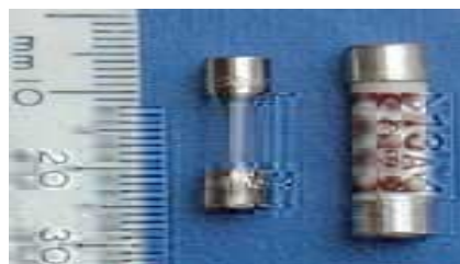
Fig5.5.2: 20 mm 200 ma glass cartridge fuse used inside equipment and 1 inch 13 A ceramic British plug fuse.
