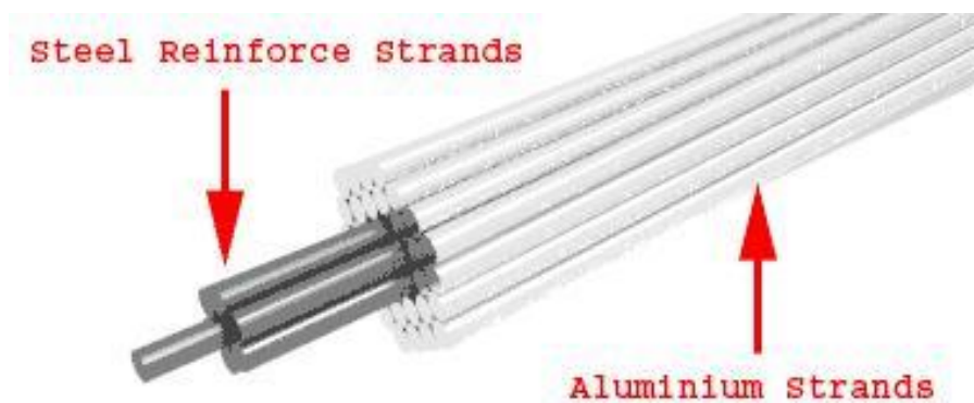
Figure 5.4 5ACSR (Aluminum Conductor Steel Reinforced)
