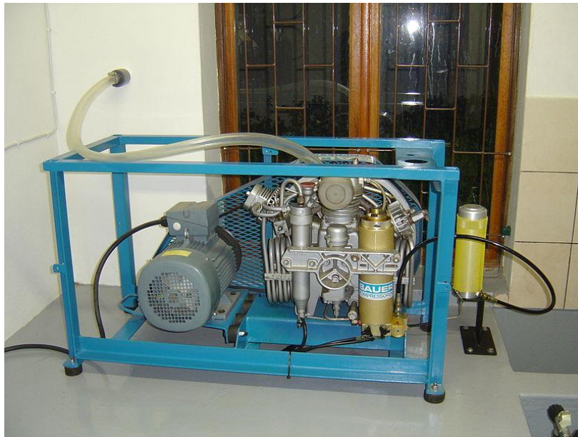
Figure 1.1 A small stationary high pressure breathing air compressor for filling scuba cylinders
