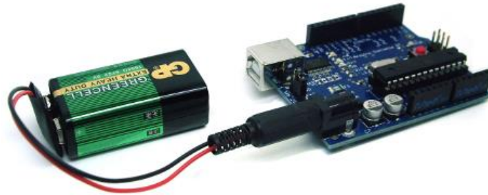
Figure 4.10: Power supply to the Arduino.
