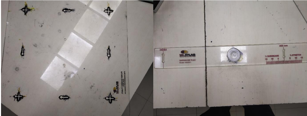
Figure 3. 1: Stability shrinkage template and shrinkage ruler
