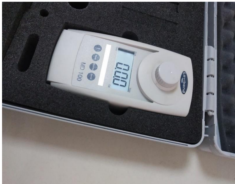
Fig.3.3: Suspended solid measuring instrument
